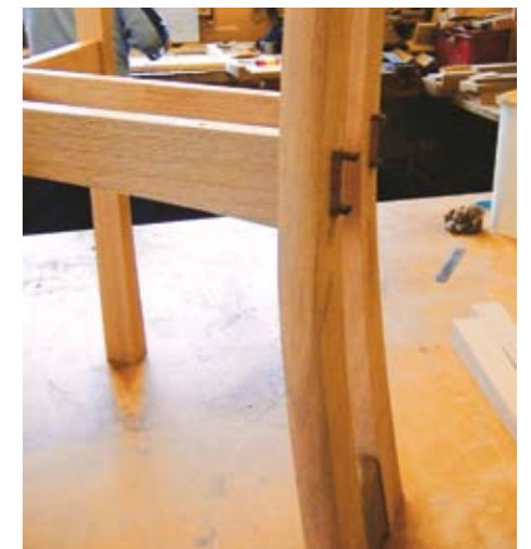
▲ The through-mortise and tenon joints were attractive, but they also provide strength
