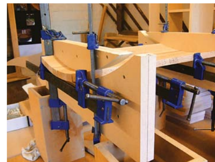
◀ The curved sides of the lectern were coopered. Getting the angles of their bottoms to fit with the curve of the base proved very tricky
