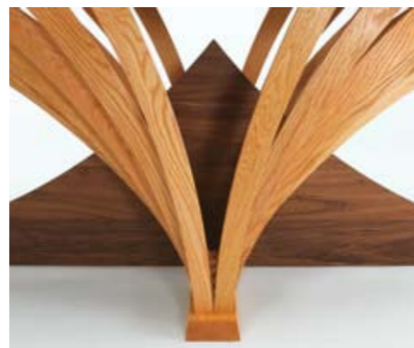
▲ The arms were secured to two rails using screws; these sit below the table-top and support it
