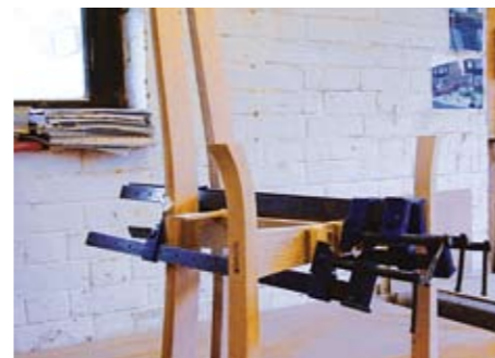
▲ The front and back leg components were shaped on a spindle moulder using templates
