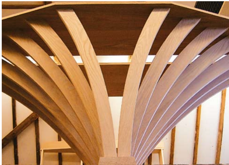
▲ The arms were secured to two rails using screws; these sit below the table-top and support it
