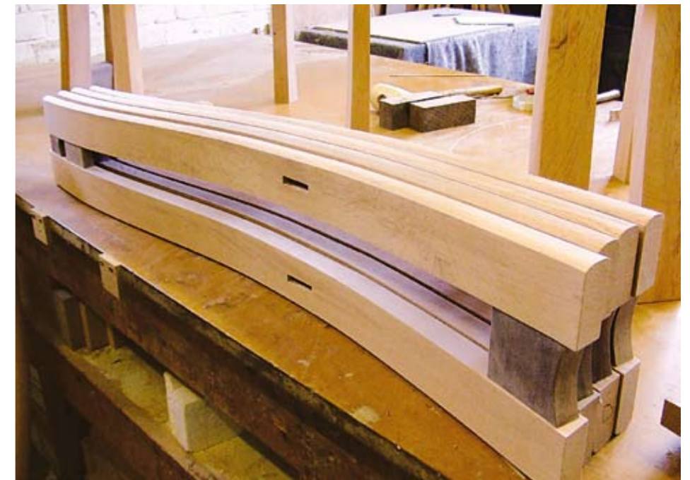
▲ The front and back leg components were shaped on a spindle moulder using templates
