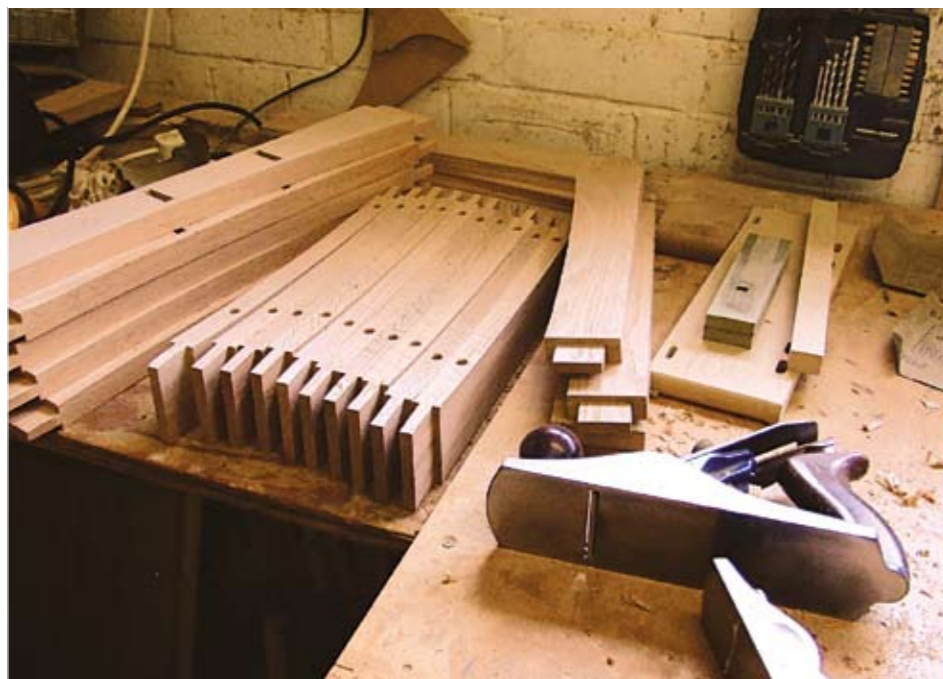
▲ With 10 chairs to make, the components were cut and jointed by batch production
